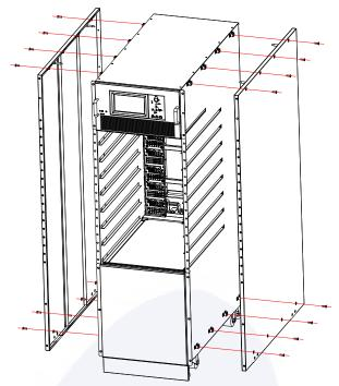
Figure 3-7 Remove the side door of the cabinet
