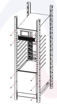
Figure 3-10 Load the UPS into the server cabinet
