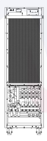
(b) 8 slot UPS Cabinet structure (back view)
