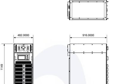
Figure 0-1 Size diagram of 6 module cabinet with PDU
