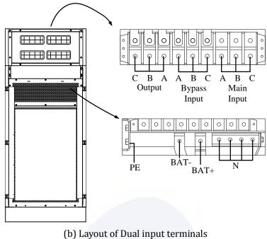
Figure 0-2 PDU Terminal layout
