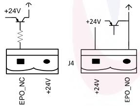
Figure 3-18 Diagram of input port for remote EPO
