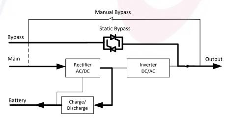
Figure 2-8 UPS conceptual diagram in ECO Mode
