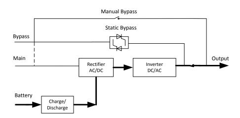
Figure 2-5 UPS conceptual diagram in Battery mode
