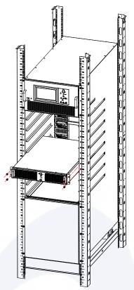
Figure 3-11 Insert module to cabinet
