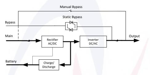
Figure 2-3 UPS conceptual diagram in normal mode
