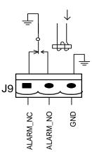
Figure 3-22 Integrated warning dry contact interface diagram
