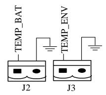
Figure 3-17 J2 and J3 for temperature detecting
