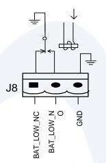
Figure 3-21 Battery warning dry contact interface diagram
