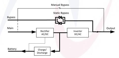
Figure 2-6 UPS conceptual diagram in Bypass Mode
