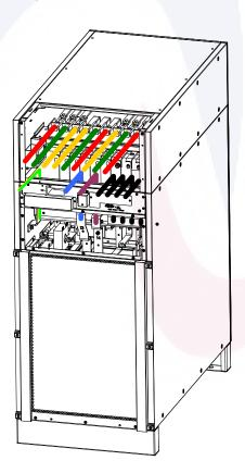
Figure 0-3 PDU Cable entry
