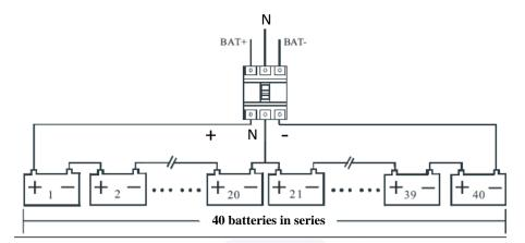
Figure 3-13 Battery string wiring diagram
