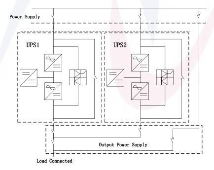
Figure 5-6 Parallel diagram
