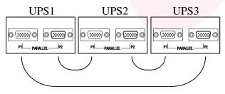
Figure 5-7 Parallel connection
