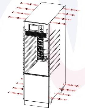
Figure 3-8 Remove bracket for cabinet side door
