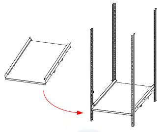
Figure 3-9 Install rack tray
