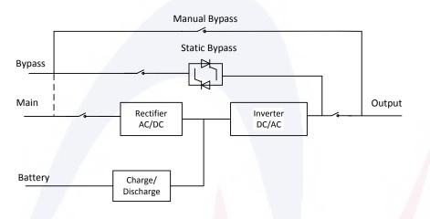
Figure 2-1 UPS Conceptual Diagram
