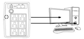
**CAUTION: NEVER** connect a laser printer or scanner to the UPS unit. This may cause the damage of the unit.
