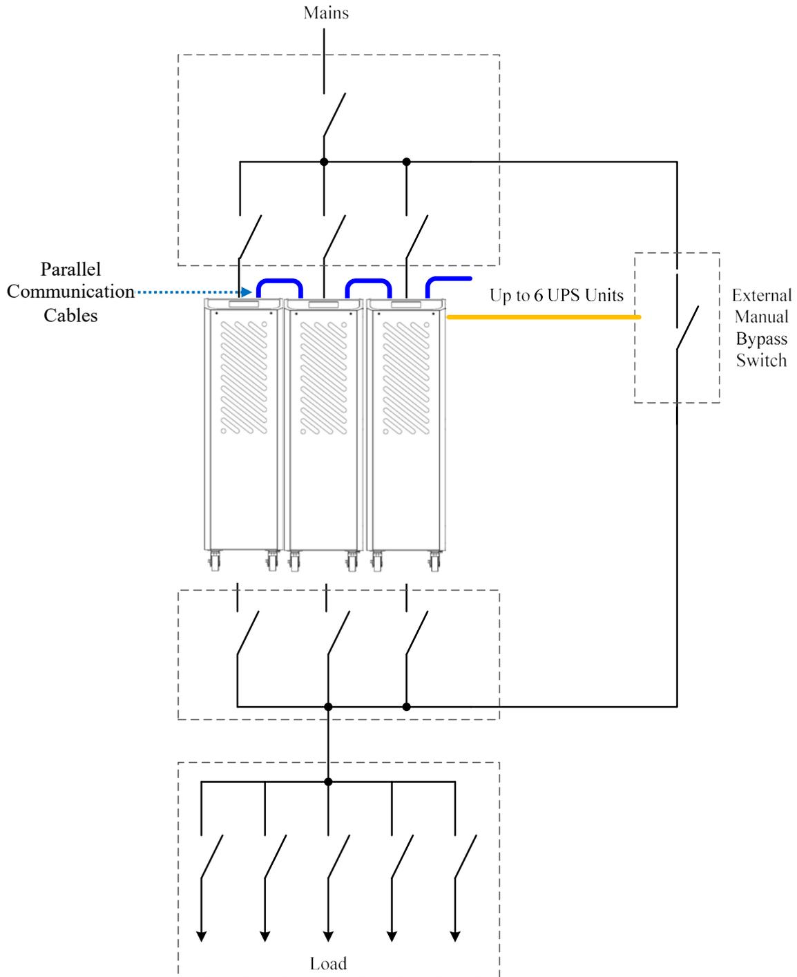
■ Recommended N+1 parallel for dual inputs system configuration
