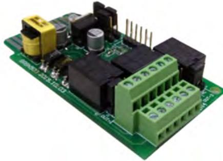
This card provides three output dry contacts and three input contact. These contacts are programmable and user can change the definition for each contact. Please refer to Dry Contact Card manual for more detail.
