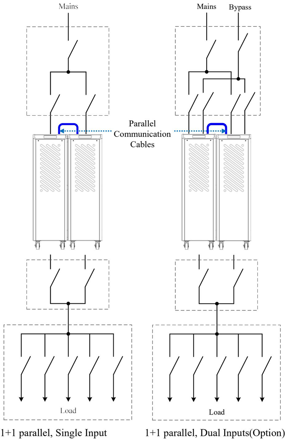
■ Recommended N+1 parallel for single input system configuration
