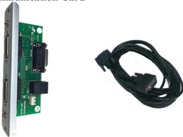
The parallel communication cards are required when UPS in parallel and it comes with 1.5 meters parallel communication cable. A longer parallel communication cable is available for more UPS in parallel.
