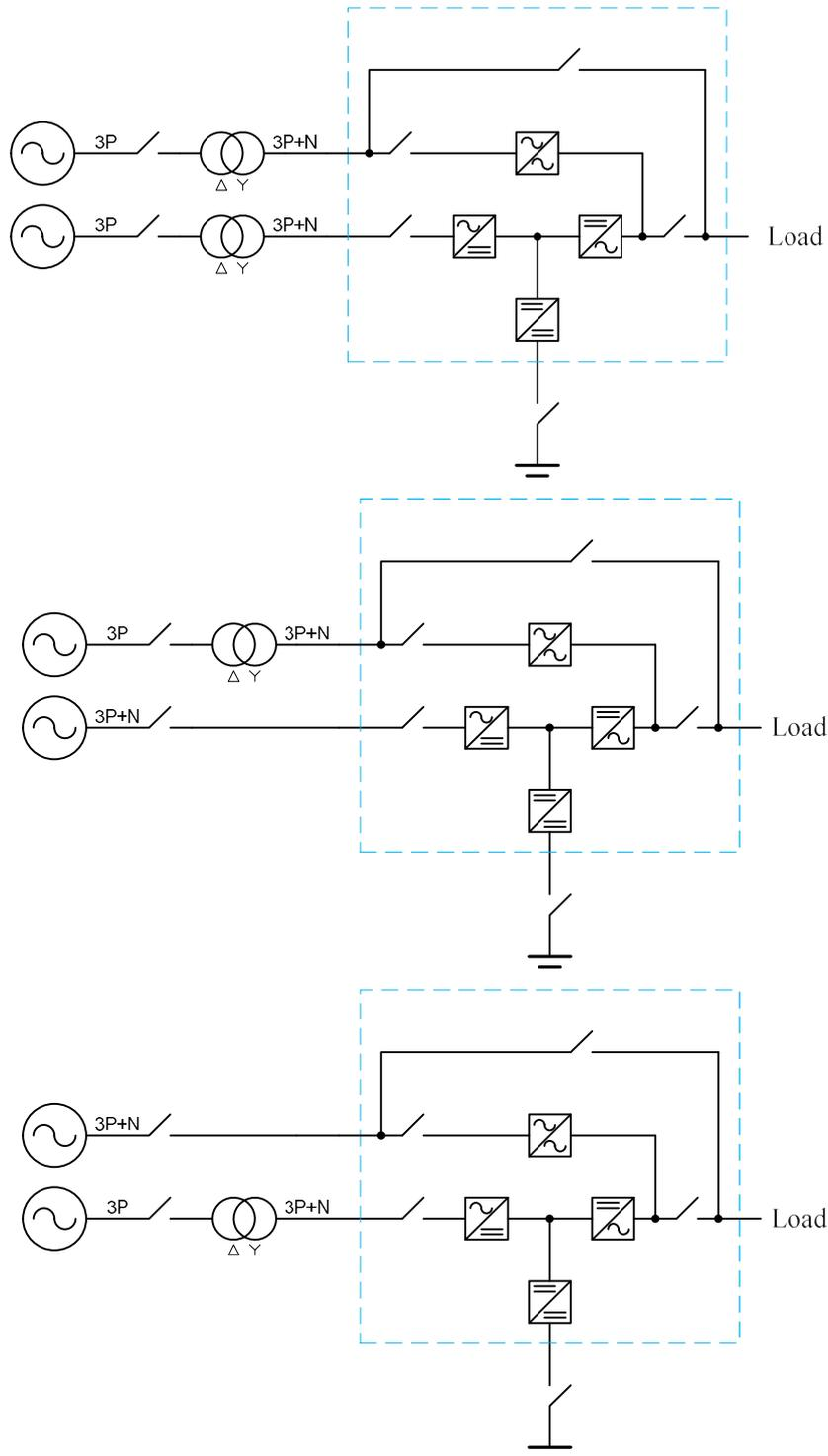
**Note :** You have to install an isolation transformer on one of the inputs if the two power system are different.
