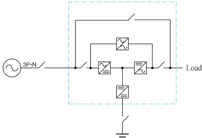
● **UPS with single input and isolation transformer**
