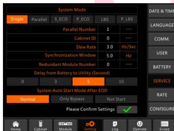
The setting interface for the parallel system
