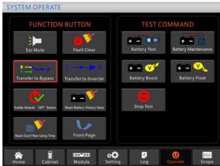
The operation interface for transferring to bypass
