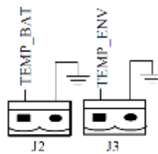
Figure 2-20 J2 and J3 for temperature detecting
