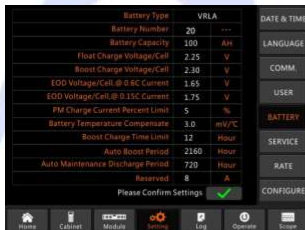
Figure 4-4 setting the period for battery auto discharge
