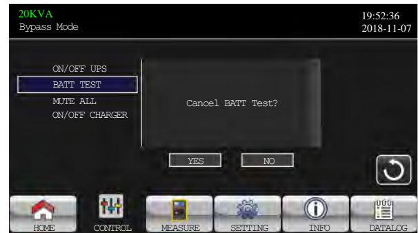
Cancel Battery Test
