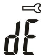
Step 3: Please press the “Enter” button (↵) to enter the settings to set the photovoltaic array as standard or parallel connection mode. Use the “Up” button (▲) and “Down” button (▼) to change between standard or parallel connection mode, which shows individually as Figures P1 and P2 below.
