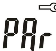
Step 4: Please press the “Enter” button (↵) to enter settings for the photovoltaic inverter machine number. The SET and ID will take turns to display on the panel at this time, which shows individually as Figures O1 and Q below. Use the “Up” button (▲) and “Down” button (▼) at this time to change the machine number setting.
