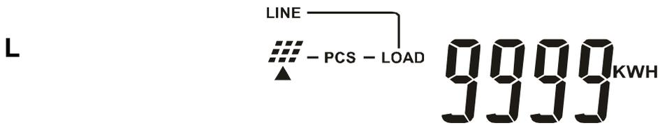
When the accumulated power generation capacity exceeds 10000KWH, the power generation capacity information will be displayed with rotation; for example when the accumulated power generation capacity is 99999KWH, it will be as shown in Figure L1 and L2.
