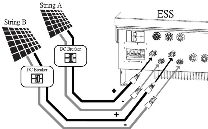
2. **Parallel connection mode:** When a single string of photovoltaic array is connected to string A and String B, users must enter setting mode to make modifications as shown in the figure below. (The setting mode is explained in Chapter 3-1-3.)
