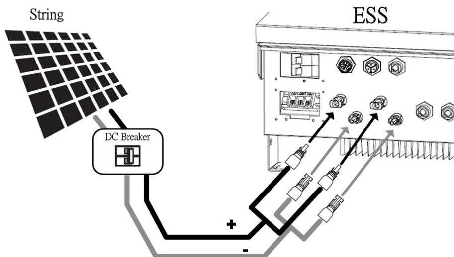
■ Recommended PV panel input wiring wire diameter
