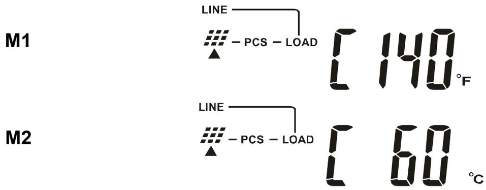
The heatsink temperature can be displayed in Celsius or Fahrenheit, as shown in Figure N1 and N2.
